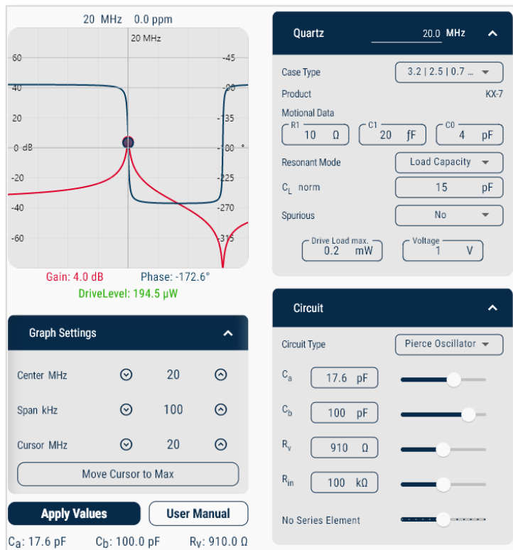
Figure 15 Pierce oscillator with asymmetrical choice of C_a and C_b (18/110 pF)
