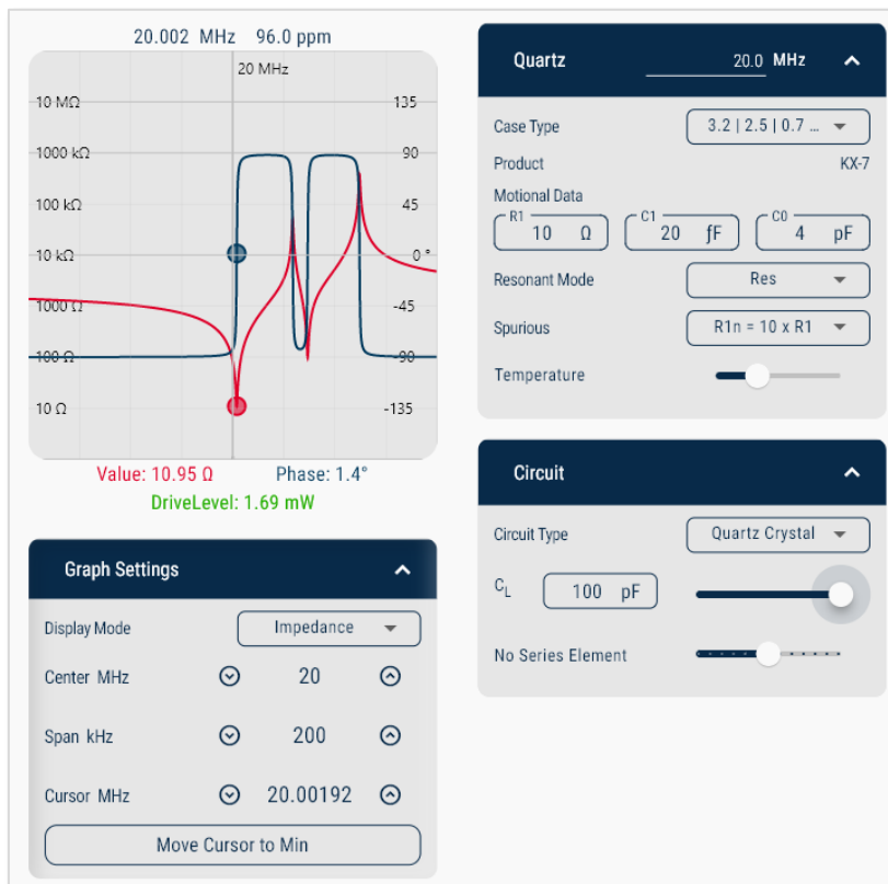
Figure 12 Series resonant quartz crystal with spurious resonance
