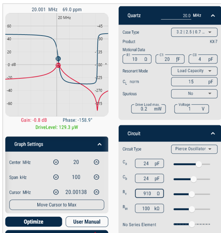
Figure 16 Pierce oscillator with symmetrical choice of C_a and C_b (24/24 pF)
