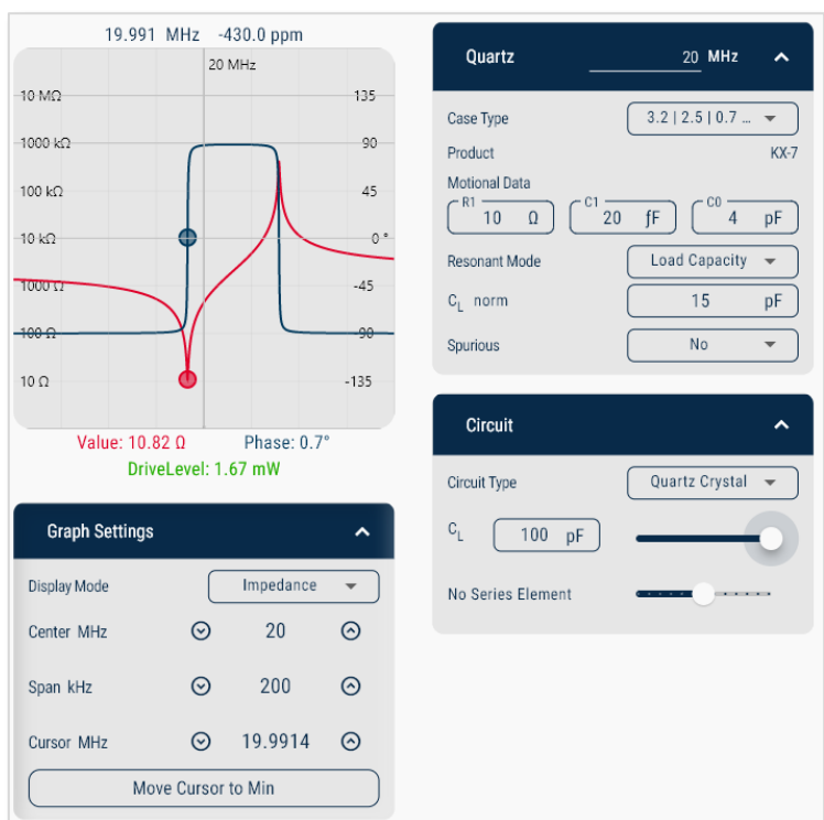
Figure 11 Quartz crystal with load) capacitance Position of load resonant frequency f_L and series resonant frequency f_S
