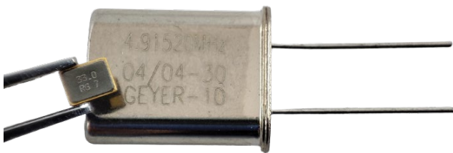
Fig 1: A modern SMD crystal over a quartz of the older design "HC-49" (3.2 x 2.5 mm or 13 x 10 mm). The volume for the accommodation of the quartz disk is much smaller. This has consequences for the electrical properties, which must be taken into account. (GEYER Electronic)
