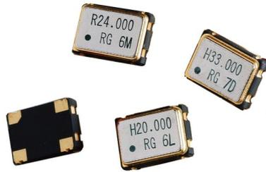
Pic. 1: SMD crystal oscillator with a size of 7 x 5 mm. Such oscillators are available for a frequency range of 1 MHz to 160 MHz and for supply voltages of 1,8 V / 2,5 V / 3,0 V / 3,3 V and 5 V. (GEYER ELECTRONIC)
