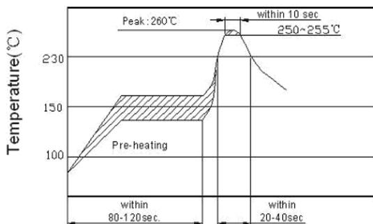
Reflow of high soldering temperature district: 260°C max., 10s max.
