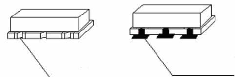
The metallic part should be soldered fully otherwise the part may be fallen off
