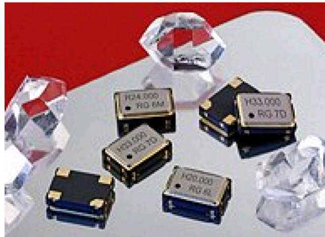
Pic. 1: SMD crystal oscillator with a size of 7 x 5 mm. Such oscillators are available for a frequency range of 1 MHz to 160 MHz and for supply voltages of 1,8 V / 2,5 V / 3,0 V / 3,3 V and 5 V. (GEYER ELECTRONIC)
